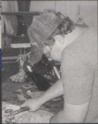
After welding, Jamie Keener bends the hot metal.
